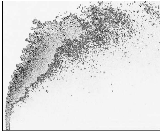
Figure 3.4: The original image with the results superimposed. Image 216001a, Case 19, p=2 bars, T=200^{\circ}\text{C} , V_{\text{Jet}}=38 m/s, and V_{\text{Air}}=93 m/s.
